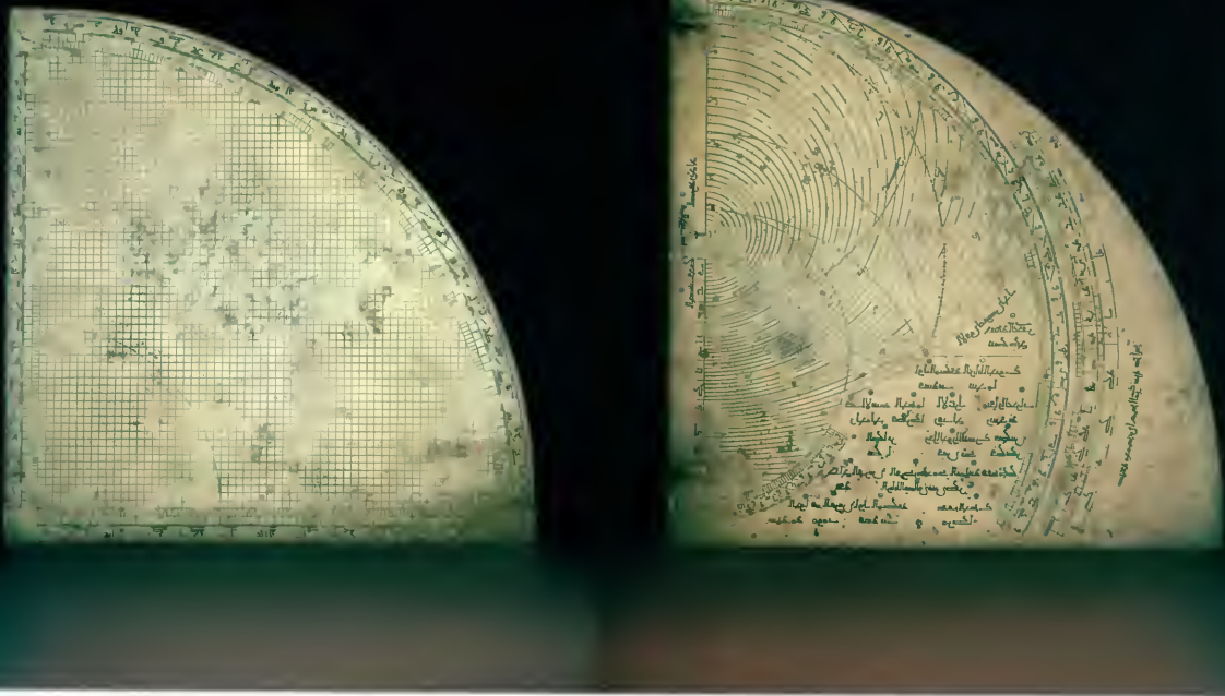
Reverse and obverse of a 14 th -century astrolabic quadrant made by Ibn Ahmad al-Mizzi, the official time-keeper of the Great Umayyad Mosque in Damascus, Syria.
